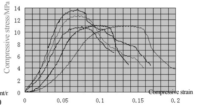
Fig7 Hollow stalk specimen’s stress - strain curves
