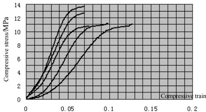
Fig8 Fitted curves of stress - strain curves of hollow specimen
