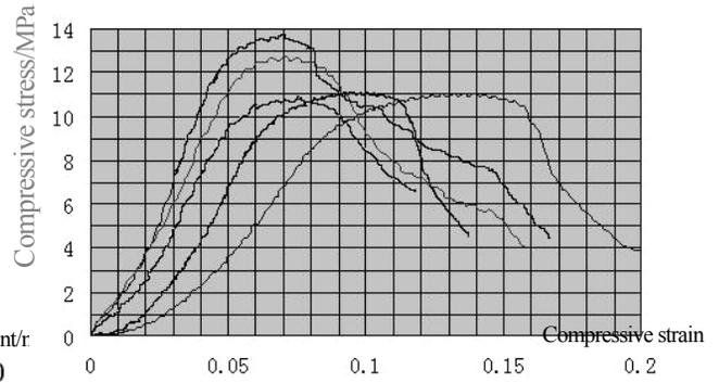
Fig7 Hollow stalk specimen’s stress - strain curves
